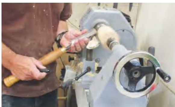
▲ Pic.4 The tool is presented to the wood with the right hand down and the tool tucked into your body
